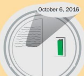
A white smoke alarm is shown with a date stamp 'October 6, 2016' and a green battery icon, indicating the date of manufacture and battery status. | <p><b>2</b> Look at the back of the alarm for the date of manufacture.</p>                 |
